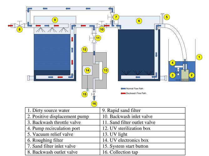
Figure 2: Aguilar BYOW System Schematic
