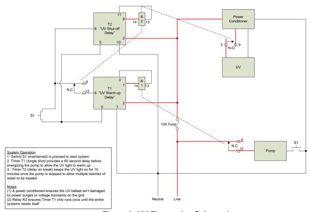
**Figure 3: UV Electronics Schematic**
